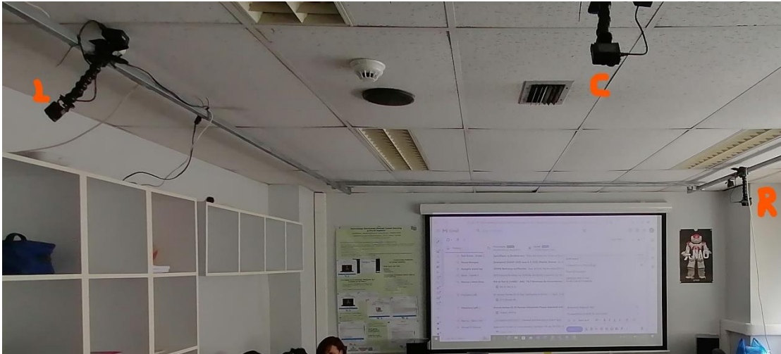
Figure 2: Evaluation room with GoPro setup. L indicates left side camera, C indicates central camera, R indicates right side camera.
